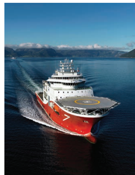
Subsea 7's Seven Falcon is one of the most advanced diving vessels in the world, featuring a 24-man twin bell saturation diving system rated to 400m and equipped with a Kongsberg K-POS DP 21 with back-up K-POS DP11.
