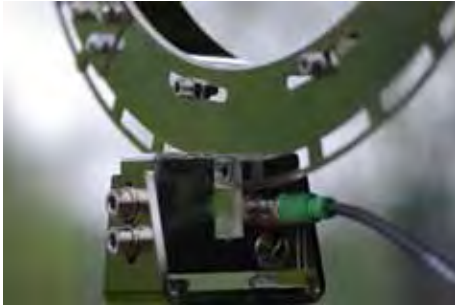
Kongsberg MetaPower® system, optical sensors installed on the rotating shaft
