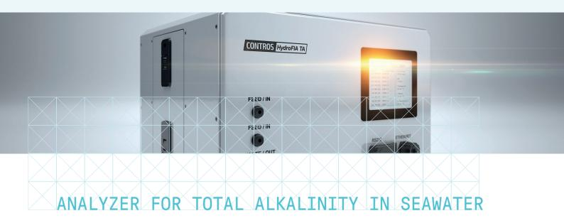
The CONTROS HydroFIA® TA is a flow through system for the determination of the total alkalinity in seawater. It can be used for continuous monitoring during surface water applications as well as for discrete sample measurements. The autonomous TA analyzer can be easily integrated into existing automated measuring systems on voluntary observing ships (VOS) such as FerryBoxes.
