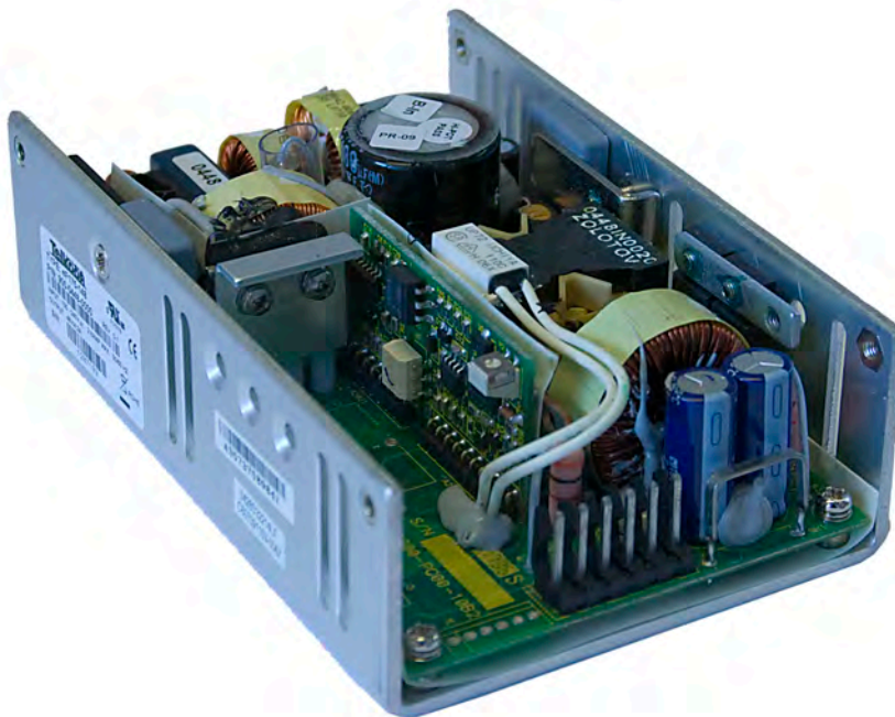
Figure 21 48 VDC power supply
