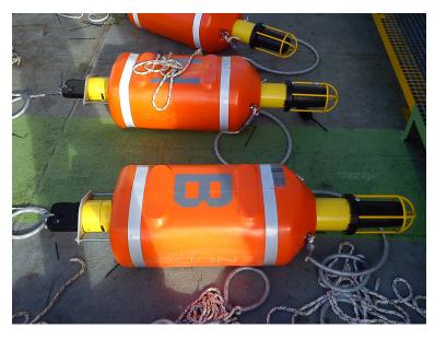
The transponders are rated to 4000 m with a housing made of coated anodised aluminium or stainless steel. The transponders are designed with a modular construction which means that the transducer, transponder electronics, battery pack and optional add-on's can be replaced individually to suit the operation.
