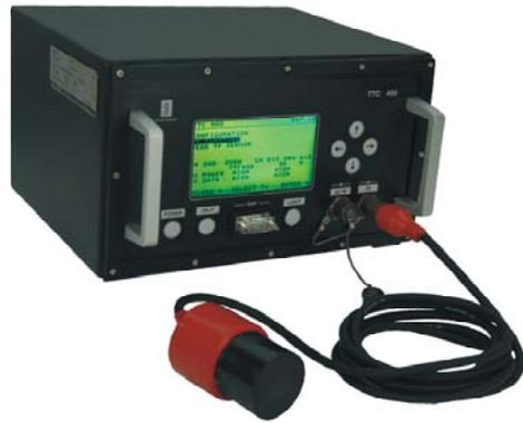
The TTC 400 is normally used for test and configuration of a transponder on deck.
