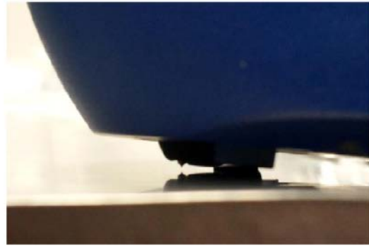
Figure 73 - Curvature causing stylus to leave surface
