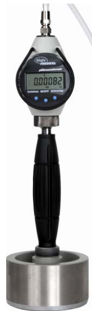
Figure 43 - Air Gauge (Mahr)
