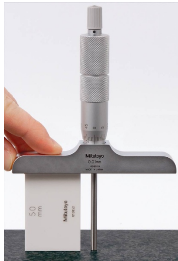
Figure 27 - Checking Depth Micrometer with Gauge Block (Mitutoyo UK Ltd)
