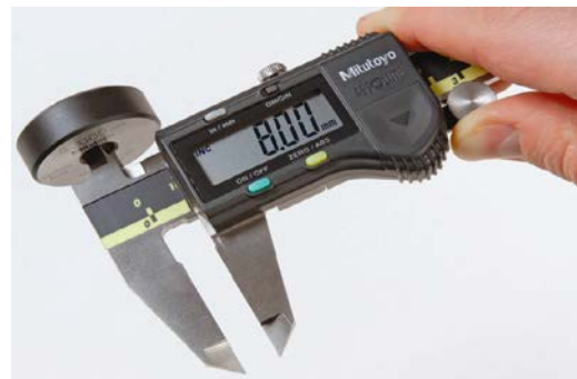
Figure 20 - Checking Anvils with Setting Ring (Mitutoyo UK Ltd)
