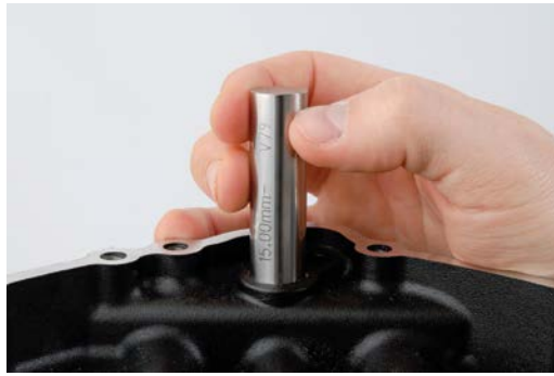
Figure 63 - Using the Plug Gauge (Mitutoyo UK Ltd)
