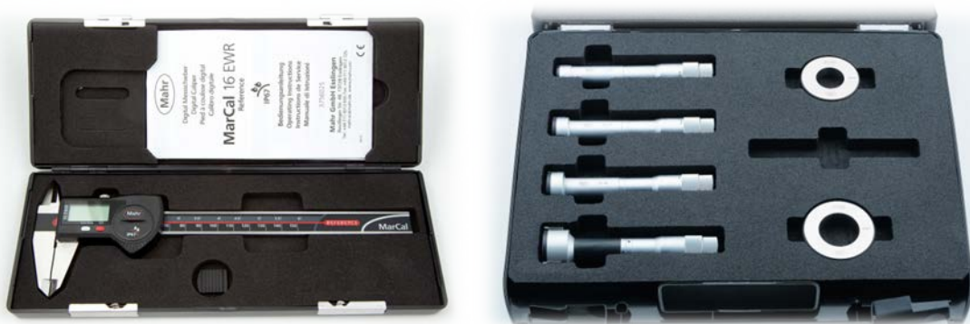
Figure 6 - Good gauge storage practice
