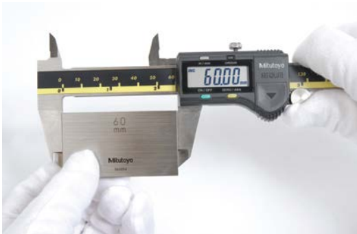
Figure 19 - Checking Anvils with Gauge Block
