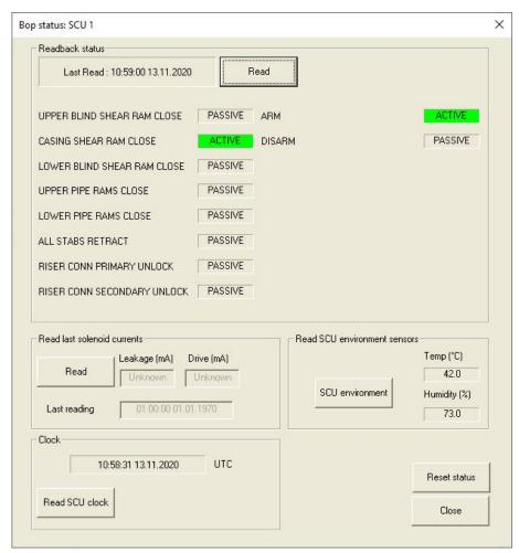
This group of functions is used to show an overview over the status (active/passive) of all digital readbacks.
