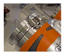
7 Insert the locking cord by pushing it sideways around the body.
