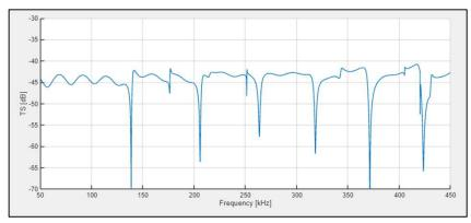
The theoretical frequency response of the WC25 mm calibration sphere is plotted. The plot is calculated by MacLennan (1981), "The theory of solid spheres as sonar calibration targets", using salt water with a sound velocity of 1480 m/s.
