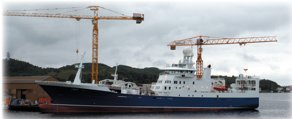
F/V Libas is a modern Norwegian fishing vessel equipped with a six-frequency EK60 system as well as SP70 and SH80 sonars. All systems collect data for the Institute of Marine Research in Bergen, Norway. (Photo by Jørn Grønland)
