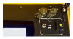
The **ON/OFF** switch is located on the right, labelled ON OFF. The LED battery level indicator is next to the **ON/OFF** switch.
