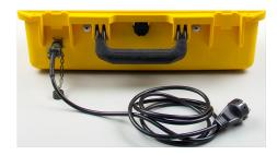
3 Connect the power cable to a 110/230 VAC power supply. Check the LED battery level indicator from time to time during charging and stop charging when it is all green.
