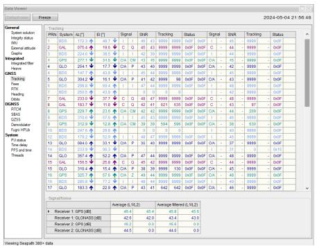
Figure 2 If right column for Signal, Snr, Tracking and status for receiver 2 is empty (as in this figure), receiver 2 is a single frequency receiver.
