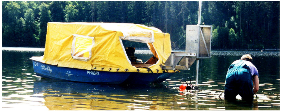
Freshwater “research vessel” with makeshift transducer mount
