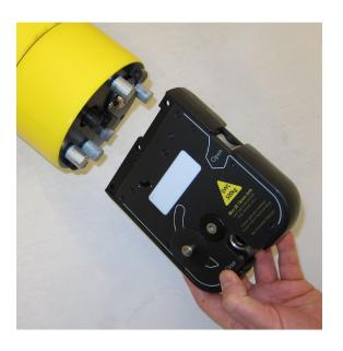
4. Remove the Hook unit. You may have to wiggle or tap gently the unit with a hammer to release a jammed unit.
