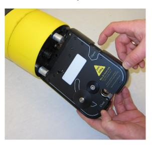
6. The mechanism operates by slowly rotating the off-center shaft that can be seen when the Hook unit is removed.
