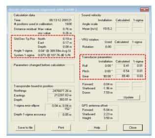
The calculated installation parameters should be very close to the old values if the alignment is a verification. If some values have changed significantly, it indicates changes to the reference sensors (motion sensor/gyro) or a potential problem with the transducer. For the transducer, it can be as simple as marine growth on the transducer if it hasn't been maintained for a while.
