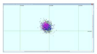
Graphic presentation of the calibration result is available through scatterplots which display measured positions and corrected positions, so it is easy to judge the quality of the logged data and effect of the new corrections.
