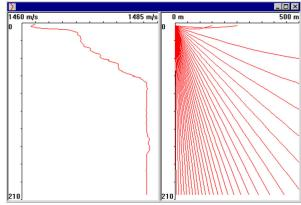
For best results of an alignment a fresh sound velocity profile of the area should be loaded into APOS so realtime ray bending compensation can be done.
