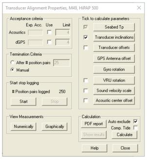
Several installation parameters can be calculated from the transducer alignment. As a rule of thumb, do not calculate parameters that are already known/measured. Calculating several parameters, and not only the transducer heading/roll/pitch will distribute the measured errors to all parameters calculated. This is why a dimensional control (or previous report) and a fresh sound velocity profile is strongly recommended.
