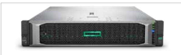
MEOS™ CAPTURE HRTG V12: 2U unit, two channels, conventional modes, SCCC and DVB-S2
