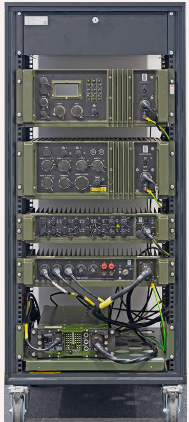
K-TaCS communication rack
