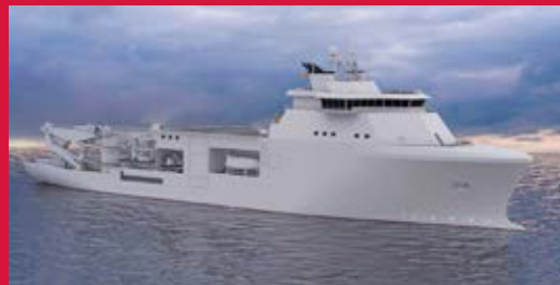
A new 120-metre Special and Diving Operations – Submarine Rescue Ship (SDO-SuRS) being built by the T.Mariotti shipyard for the Italian Navy will feature a range of Kongsberg solutions, including a pair of Elegance electric propulsion pods. The compactly designed pods have a low oil content and double barrier seal solution, to protect the ocean, while offering vessels the ability to operate in fully electric zero emissions mode in port or for limited offshore operations.
