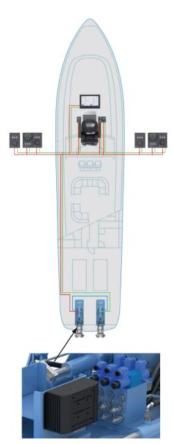
For steel- and aluminium series the controls and key hydraulic components are incorporated in the jet unit and calibrated at the factory, simplifying installation.
