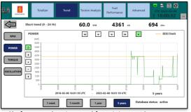
Shaft power data is stored for minimum 10 years in tamperproof database in the processing unit.
