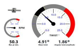
Gauge vision of twist and RPM of the coupling. The colored area(black) visualizes the current amplitude of twist oscillations.
