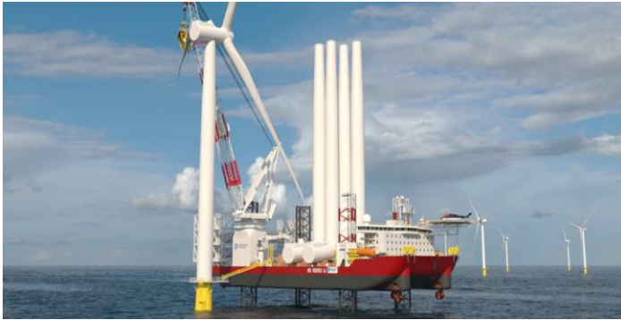
Wind Turbine Installation Vessel (WTIV) to Dominion Energy
