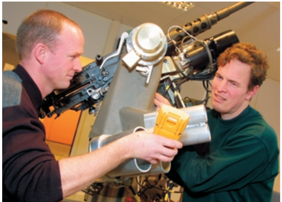
Testing weapons control systems for deployment on the armoured personnel carriers destined for the US Army.
