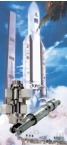
Kongsberg Gruppen makes the attachment and separation mechanism that connects the Ariane 5's main engine and boosters. Separation takes place two minutes into the flight, and must be accomplished within five milliseconds
