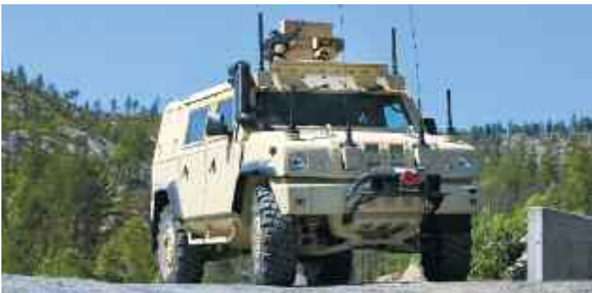
The principal underlying the Protector Remote Weapon Station is that the weapon and sensors are mounted outside the vehicle, while the operator operates them from a protected position inside the vehicle.
